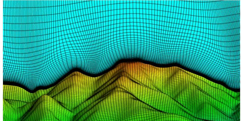
*Figure 1: Example of a computational mesh for terrain CFD simulation.*
